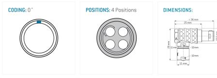
The pin layout corresponds to the view on the termination area
