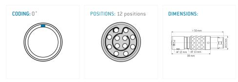
The pin layout corresponds to the view on the termination area
