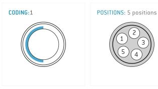
The pin layout corresponds to the view on the termination area
