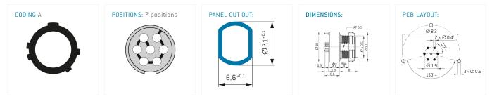
The pin layout corresponds to the view on the termination area
