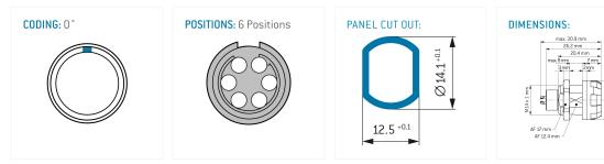
The pin layout corresponds to the view on the termination area
