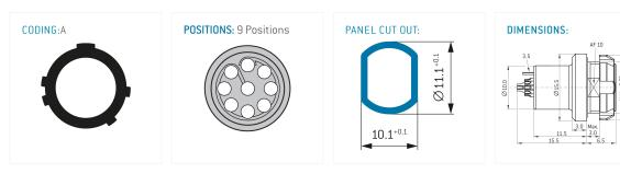
The pin layout corresponds to the view on the termination area
