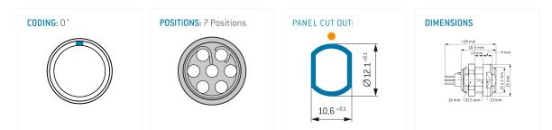
The pin layout corresponds to the view on the termination area
