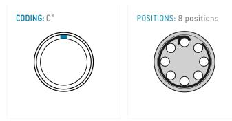
The pin layout corresponds to the view on the termination area
