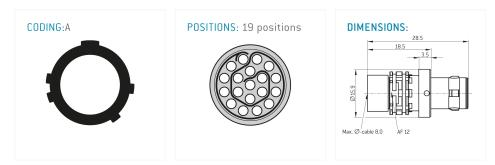
The pin layout corresponds to the view on the termination area
